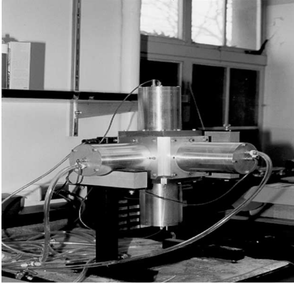
FIG. 8 Triaxial compression tester (from Kamath, 1996 ).
